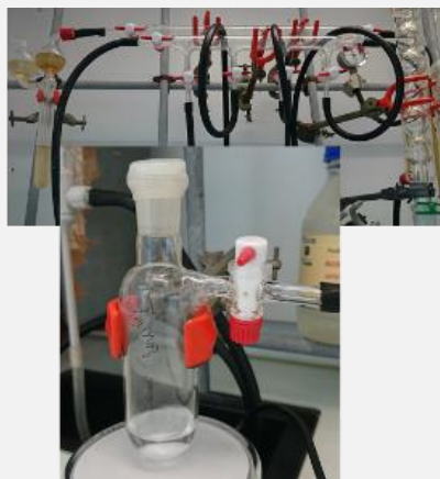
Synthesis with a Schlenk line
