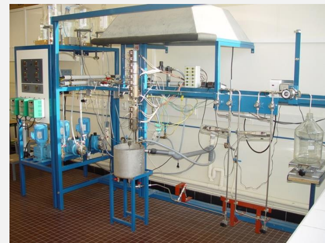
Continuous flow synthesis With Sub- or supercritical water
