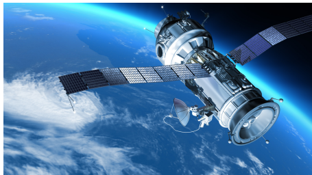
Figure 1.1: Satellite composed of a central hub and two flexible solar panels.
