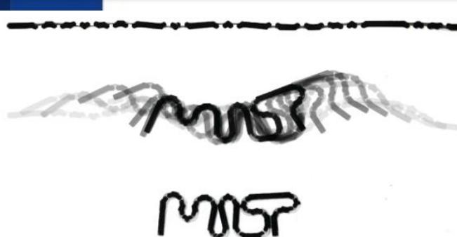
A sequence of images demonstrating the self-folding of a 4D printed multi-material single strand into the world of MIT
